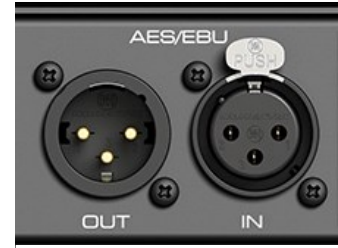
Figure 4 - AES/EBU XLR connectors
