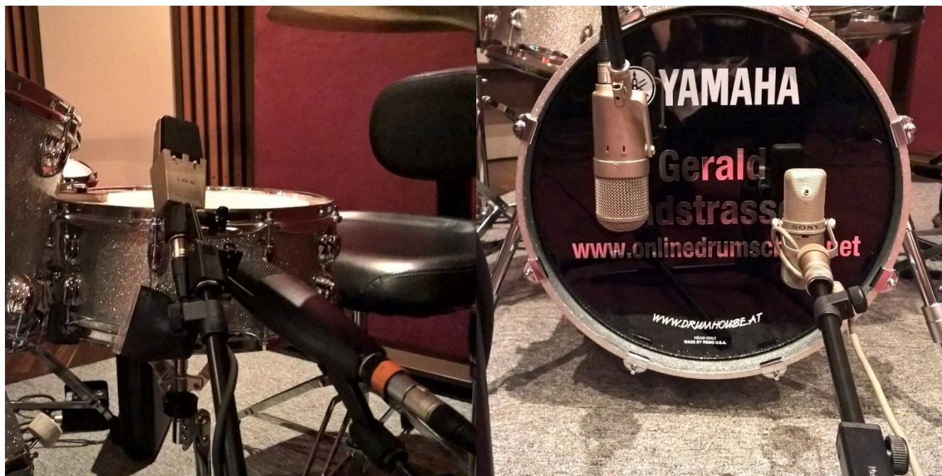
Figure 26: Snare drum, recorded with AKG C414 and Sennheiser MD421; bass drum, recorded with Neumann Fet47 and Sony C37A
