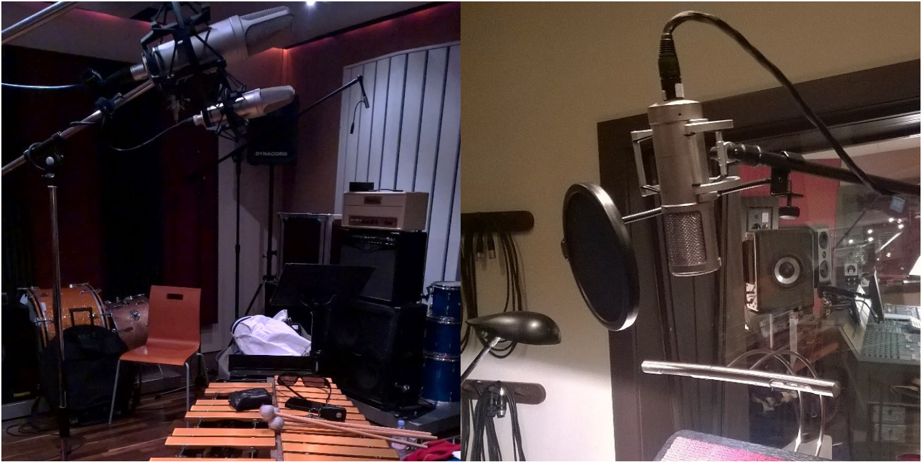
Figure 28: Vibraphone, recorded with 2 RODE NT 1000 (sort of A-B stereo); Solo Vocals, recorded with Brauner Phantom
