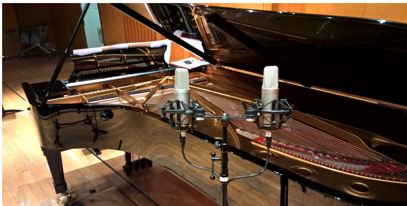
Figure 33: Steinway D grand piano, detail of the NOS stereo pair (RODE NT 1000)
