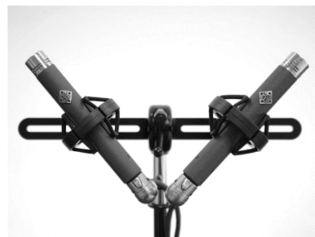
Figure 16: NOS stereo setup with Telefunken ELA M-260
