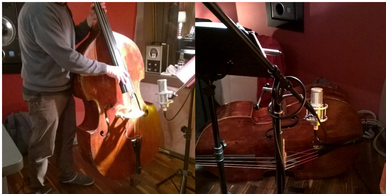
Figure 27: Acoustic bass, recorded with Brauer Phantom and internal DPA pick-up
