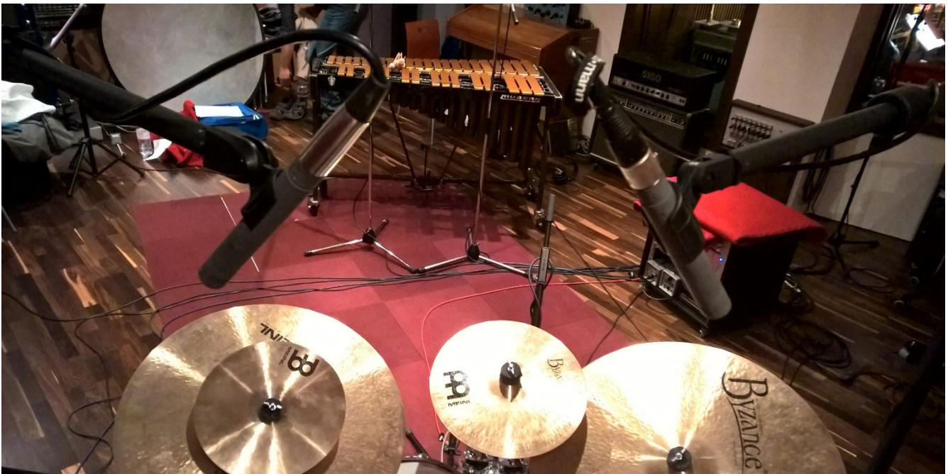
Figure 25: Drum Kit: detail of the Schoeps CMC 541 overheads in NOS configuration
