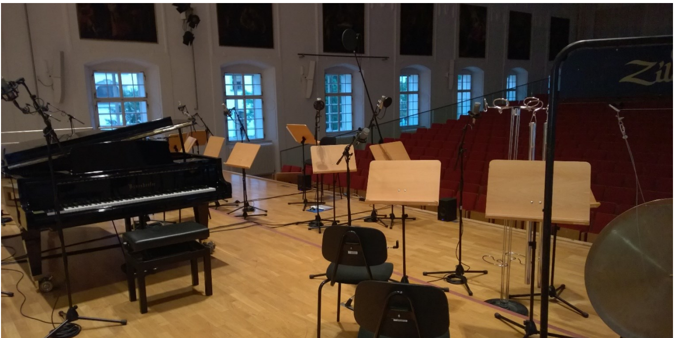
Figure 34: DNS recording setup for a mixed ensemble conducted by Albert Anglberger in the Große Universitätsaula (Salzburg), featuring OSS main stereo pair (DPA 4006), NOS for the grand piano, A-B-C-D group (NT 1000) for the children choir (on the right), 2x AT 3035 for the percussion, 4x NT 1000 for the woodwinds and the trumpet, AKG C414 for the acoustic guitar, Sennheiser MD 421 for the electric guitar amplifier, 2x Brauner Phantom for solo vocals
