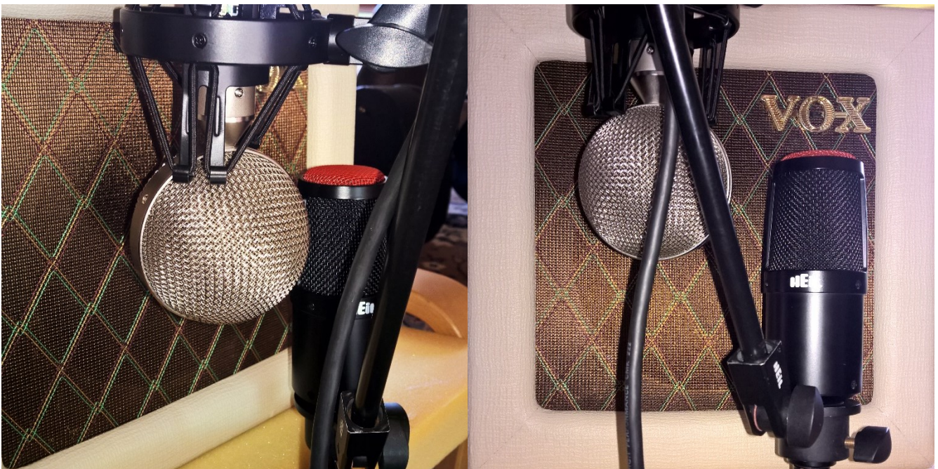
Figure 29: DNS recording: electric guitar Vox mini-amp, recorded with Cascade FatHead II (ribbon) and Heil PR-30B (dynamic) microphones
