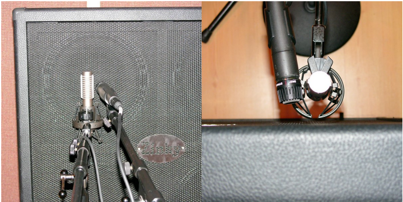
Figure 30: Electric guitar amp (with 4 speakers), recorded with Royer R-121 (ribbon) and Shure SM-57 (dynamic) microphones, both placed very close to the amp speaker cone. Source: http://www.royerlabs.com/rectips_electricguitar.html
