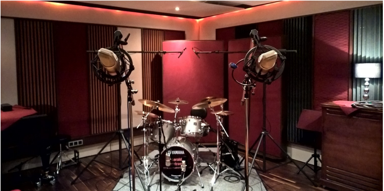
Figure 24: Jazz Drum Kit, recorded with Schoeps CMC 541 overheads (for cymbals and toms) in NOS configuration (the RODE NT 1000 are for Vibraphone)
