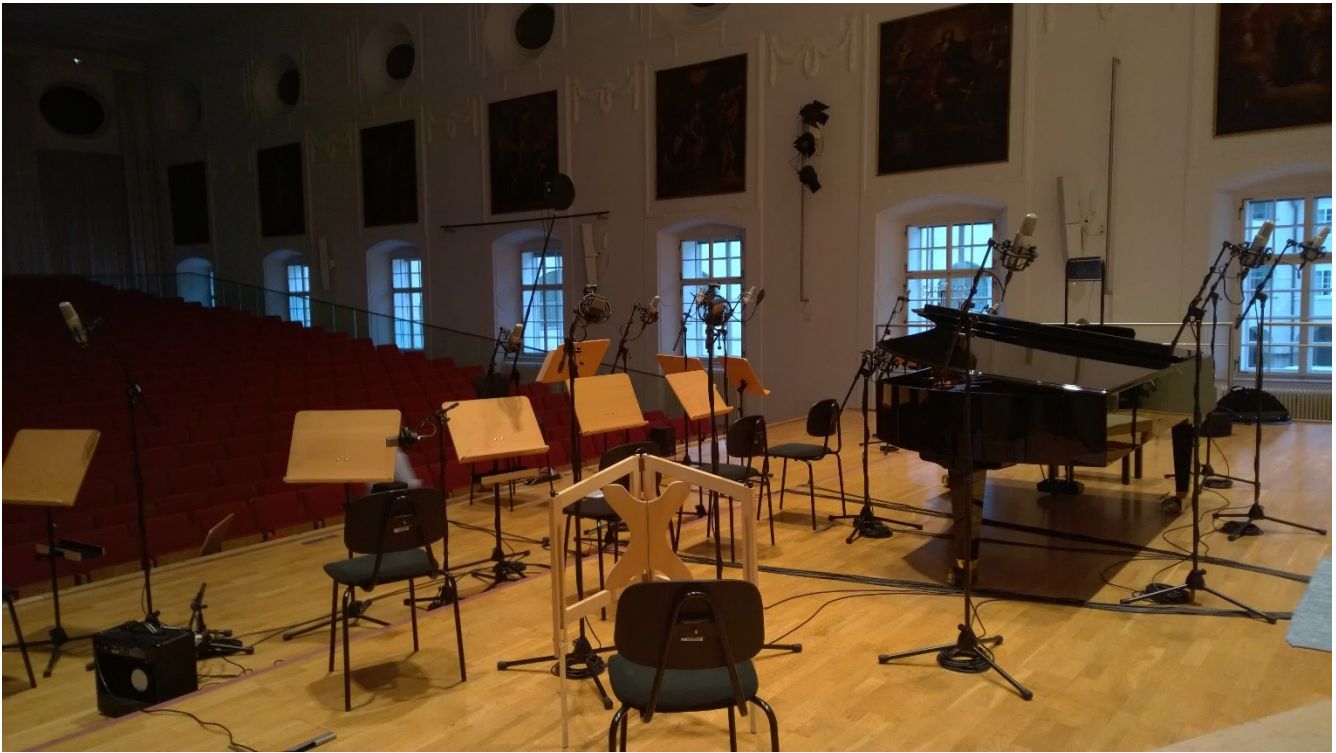
Figure 34: DNS recording setup for a mixed ensemble conducted by Albert Anglberger in the Große Universitätsaula (Salzburg), featuring OSS main stereo pair (DPA 4006), NOS for the grand piano, A-B-C-D group (NT 1000) for the children choir (on the right), 2x AT 3035 for the percussion, 4x NT 1000 for the woodwinds and the trumpet, AKG C414 for the acoustic guitar, Sennheiser MD 421 for the electric guitar amplifier, 2x Brauner Phantom for solo vocals
