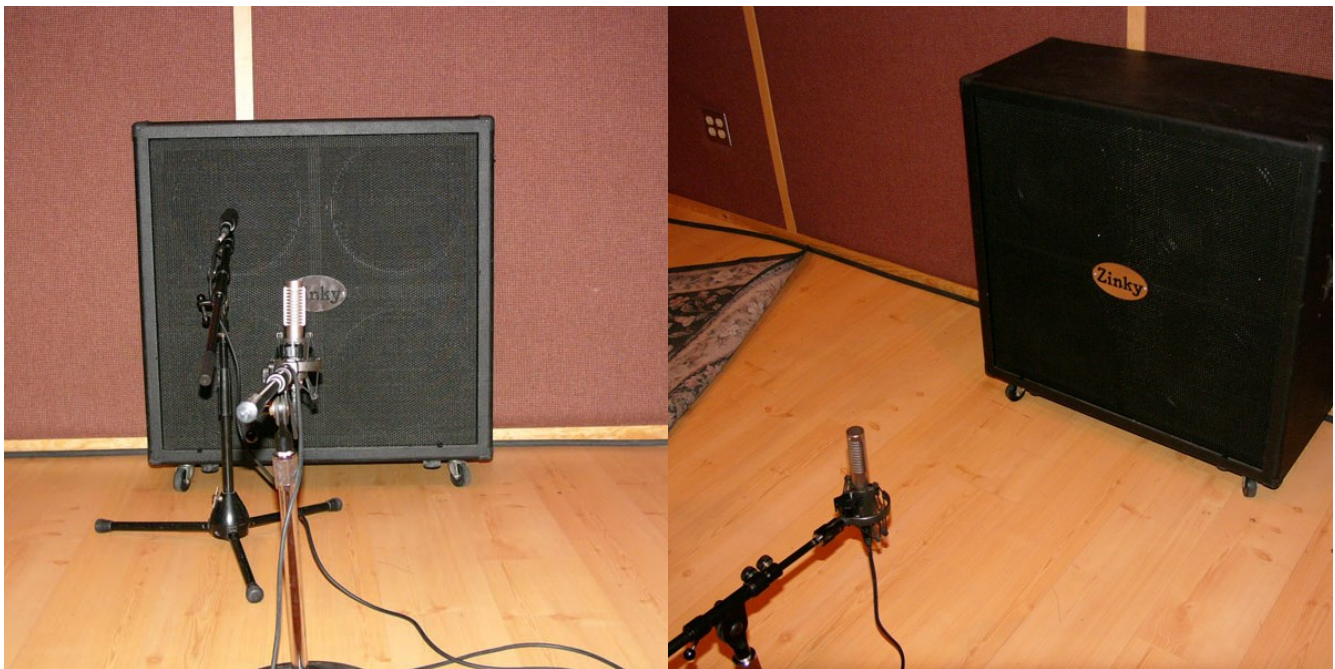
Figure 31: the same combination of amp and microphones, this time with the Shure SM-57 placed up close, and the Royer R-121 at about 50 cm distance, capturing a less direct, more “airy” sound. Source: http://www.royerlabs.com/rectips_electricguitar.html
