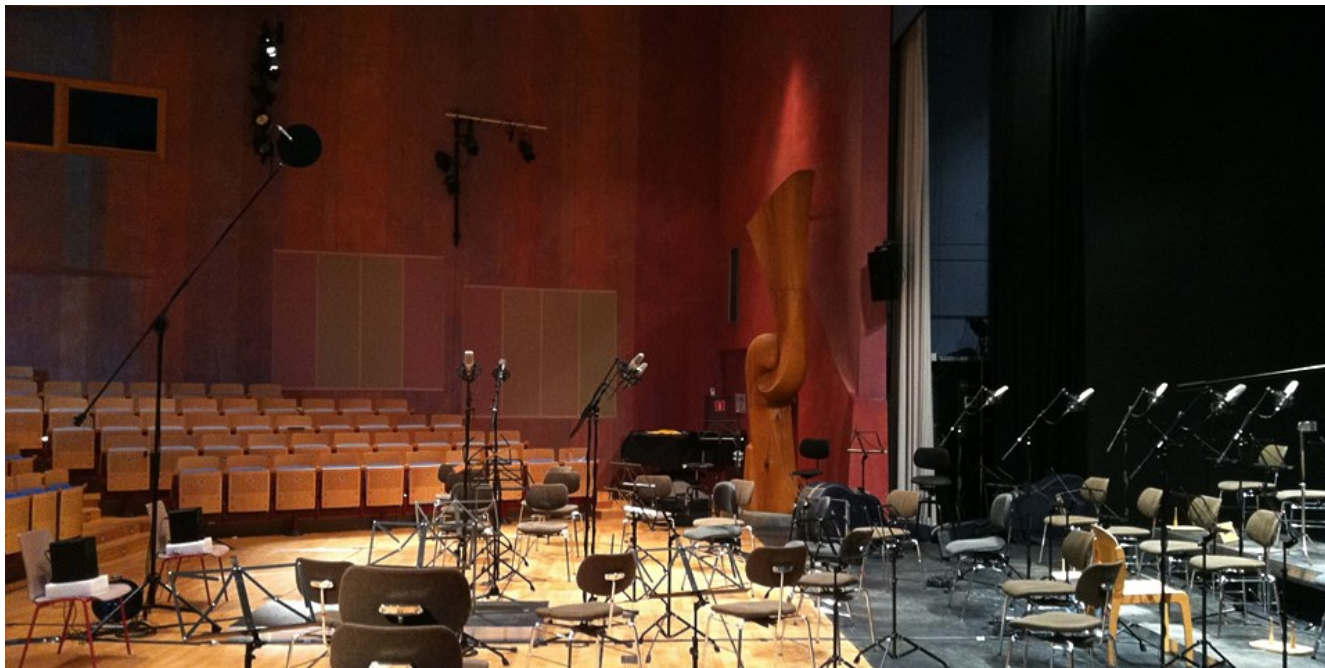
Figure 37: DNS recording setup for the Mozarteumorchester in the Odeion Saal (Salzburg), featuring OSS main stereo pair (DPA 4006 with Jecklin Disk) and 12 support microphones (RODE NT 1000, Brauner Phantom and Audio Technica AT 3035)
