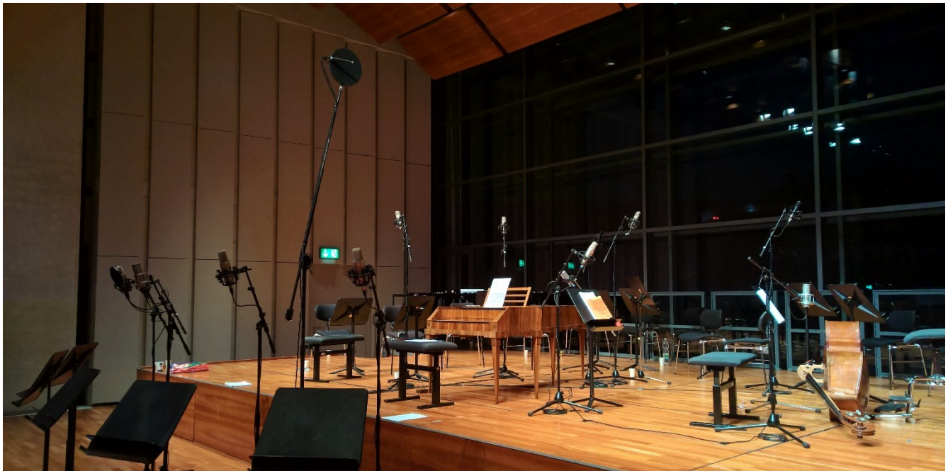
Figure 1: DNS 20-channel recording featuring: OSS main stereo pair (DPA 4006 with Jecklin Disk) and 18 support microphones (RODE NT 1000, Brauner Phantom, Audio Technica AT 3035)
