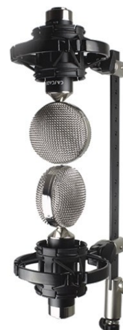
Figure 14: Blumlein stereo setup with Cascade Fat Head II
