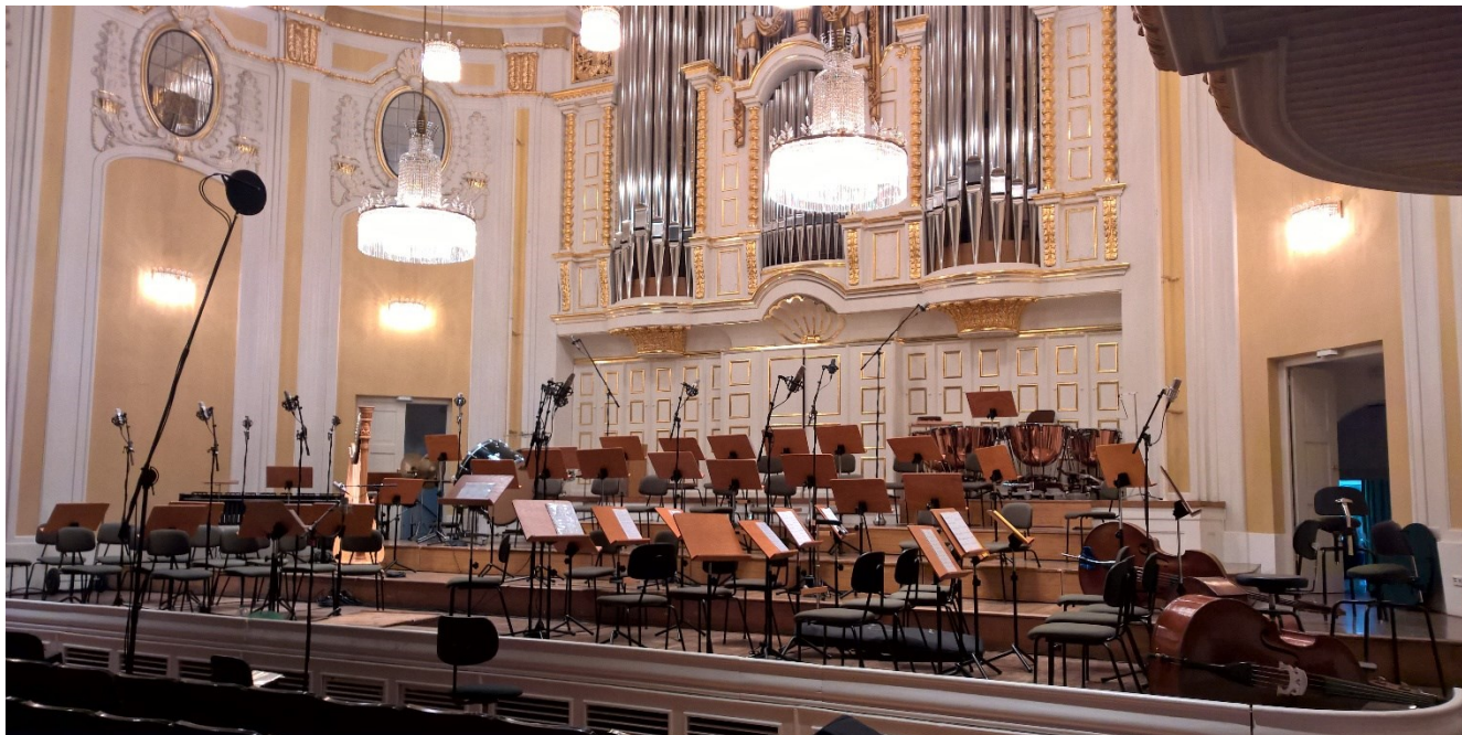
Figure 39: DNS orchestra recording setup for the Bläserphilharmonie Salzburg in the Mozarteum Grosser Saal (Salzburg), featuring OSS main stereo pair (DPA 4006) and 17 support microphones (Neumann TLM 103, AKG C414, RODE NT 1000, Brauner Phantom, Audio Technica AT 3035)
