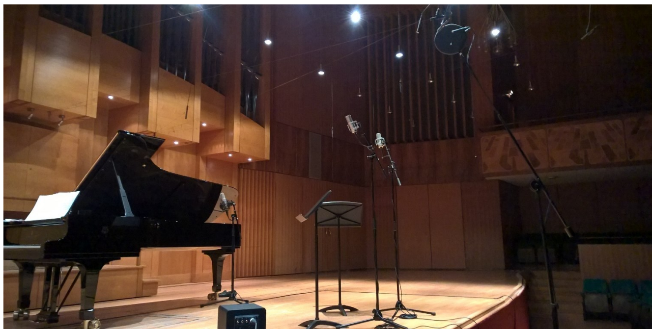
Figure 32: DNS recording, featuring a OSS main stereo pair (DPA 4006), grand piano with NOS (2x RODE NT 1000) and two violins (2x Brauner Phantom)
