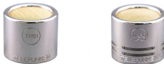
Figure 11: Telefunken TK61 omnidirectional capsule (left) and TK60 cardioid capsule (right), showing the characteristic side/rear vents (slits)
