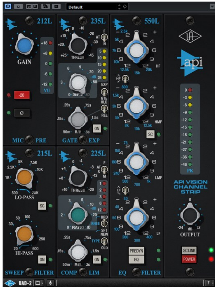
Figure 67: UAD API Vision Channel Strip (emulating API Vision console)
