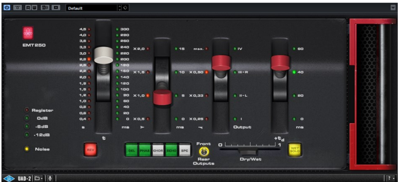
Figure 41: UAD EMT250 Digital Reverb (plugin, emulating the original hardware unit using the same algorithms)
