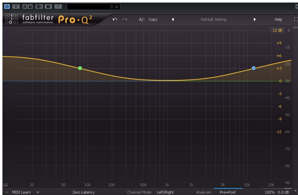
Figure 5: Low Shelving EQ set at 80 Hz (+6 dB boost) and High Shelving EQ set at 12 kHz (+6 dB boost) – FabFilter ProQ2
