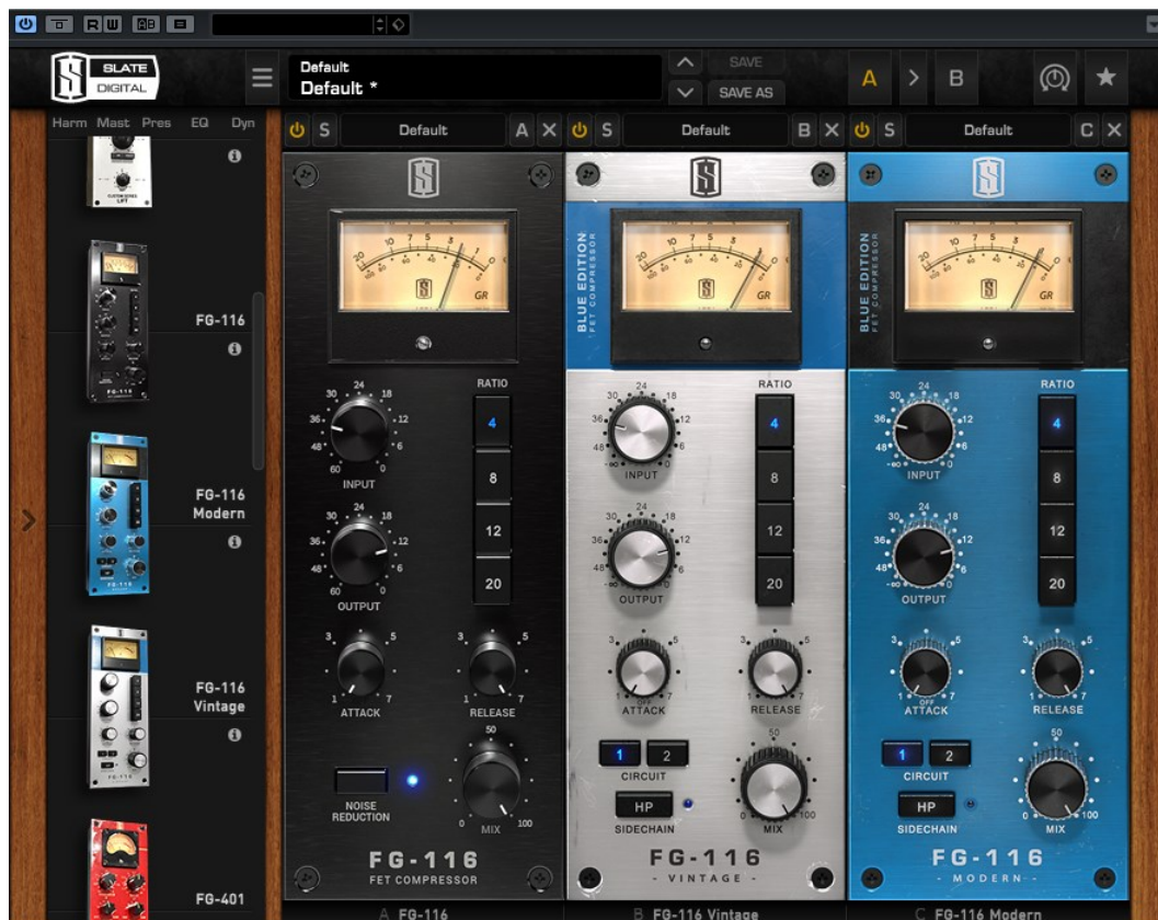
Figure 18: SlateDigital FG-116 Compressors: standard, vintage and modern (plugin, emulating three versions of the 1176LN original hardware)
