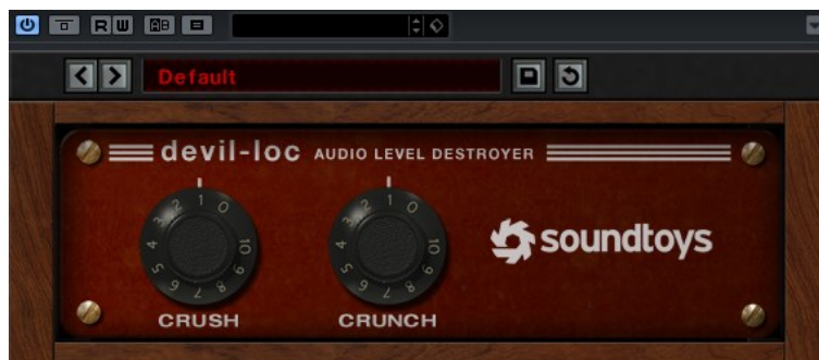
Figure 52: SoundToys devil-loc distortion (plugin, inspired by the sound of analog hardware)
