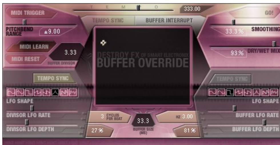
Figure 59: Destroy-FX Buffer Override, simulating a sound driver not working properly and producing several unique lo-fi effects (digital plugin)
