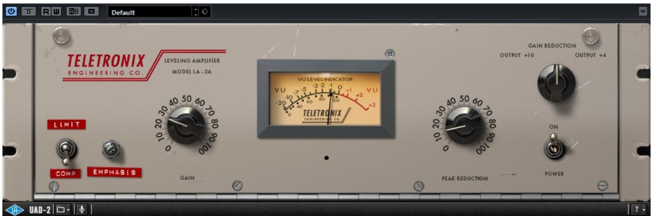
Figure 21: UAD Teletronix LA-2A opto-compressor (plugin, emulating the original hardware)
