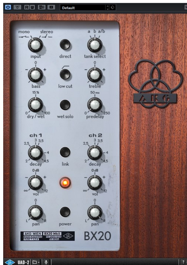
Figure 46: UAD AKG BX20 Spring Reverb (plugin, emulating the original AKG hardware unit)
