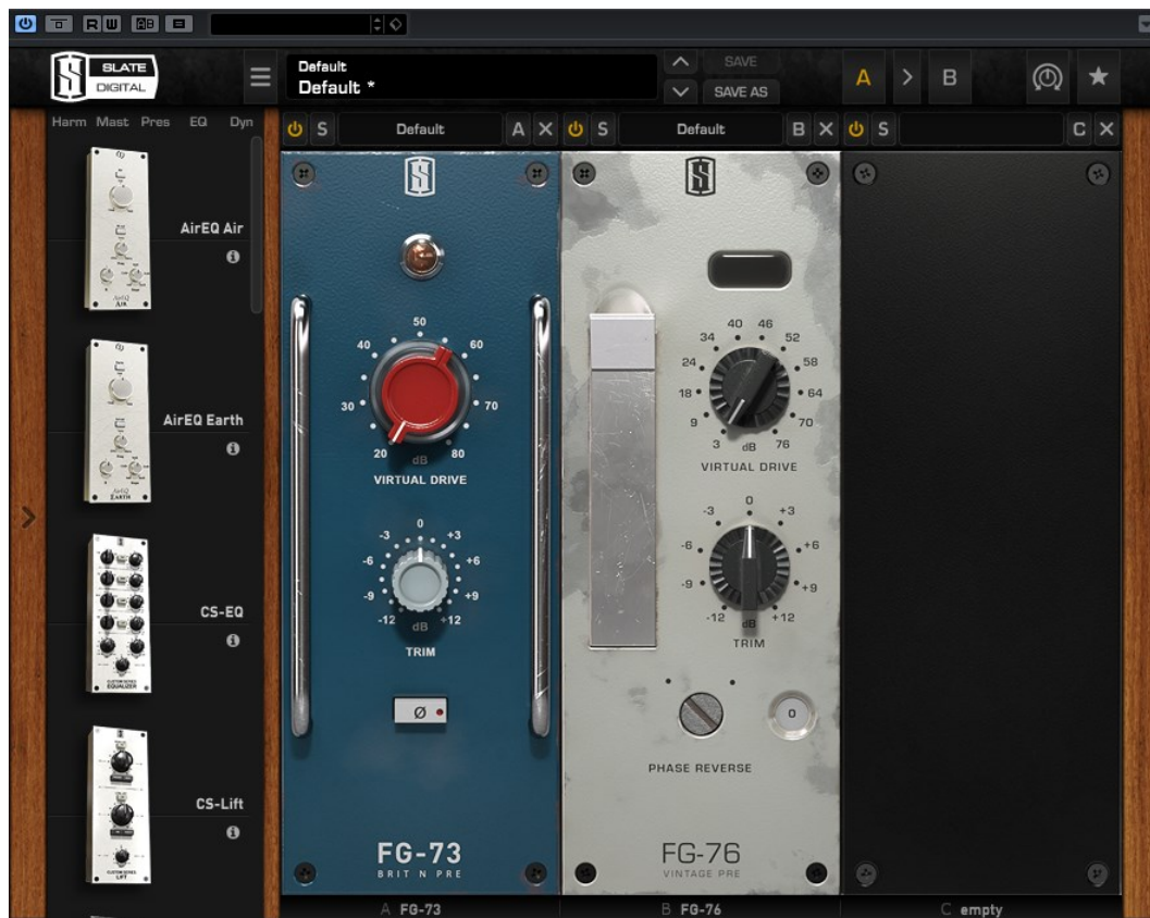
Figure 62: SlateDigital FG-73 (emulating Neve 1073 solid state preamp), and FG-76 (emulating Telefunken V76 tube preamp)
