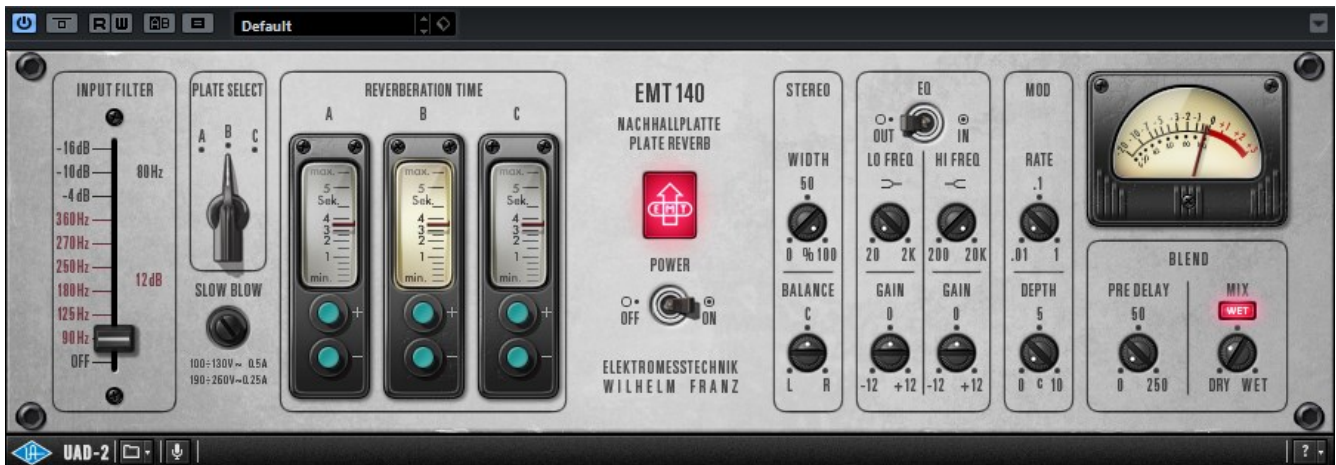
Figure 45: UAD EMT 140 Plate Reverb (plugin, emulating original EMT plate reverb hardware)
