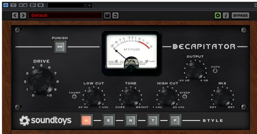
Figure 57: SoundToys 5 Decapitator Saturator (plugin, emulating the saturation of analog hardware consoles such as API, SSL, Neve, etc.)
