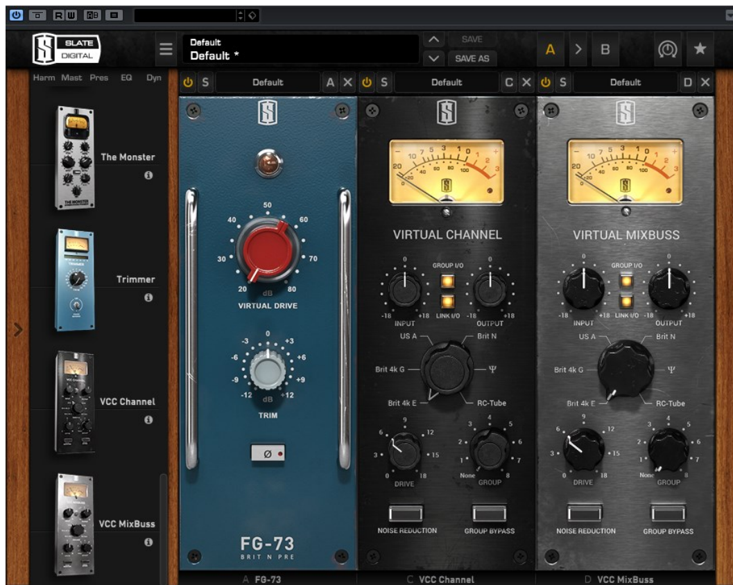
Figure 63: SlateDigital FG-73 plugin (emulating NEVE 1073 preamp), Virtual Channel and Virtual MixBuss (emulating SSL, NEVE, Trident and Tube consoles)
