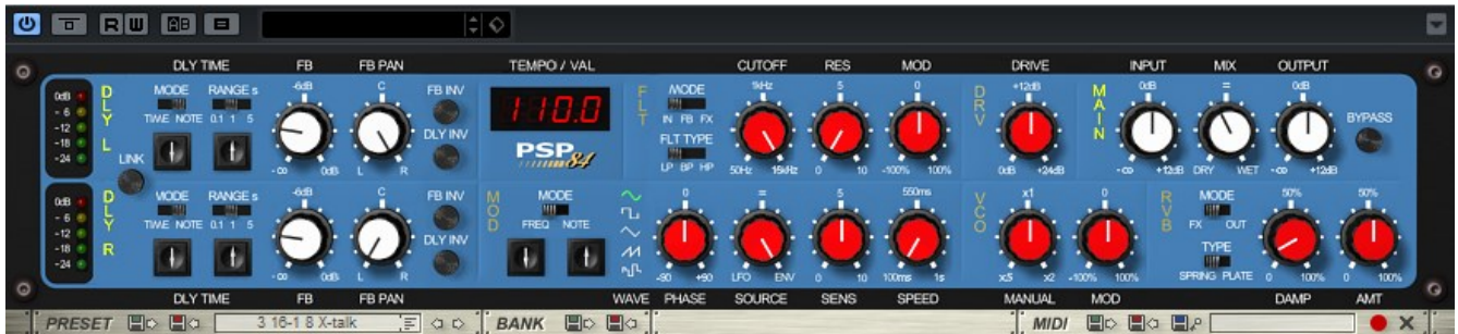
Figure 48: PSP 84 Stereo Delay (plugin, inspired by the Lexicon 42 hardware delay)
