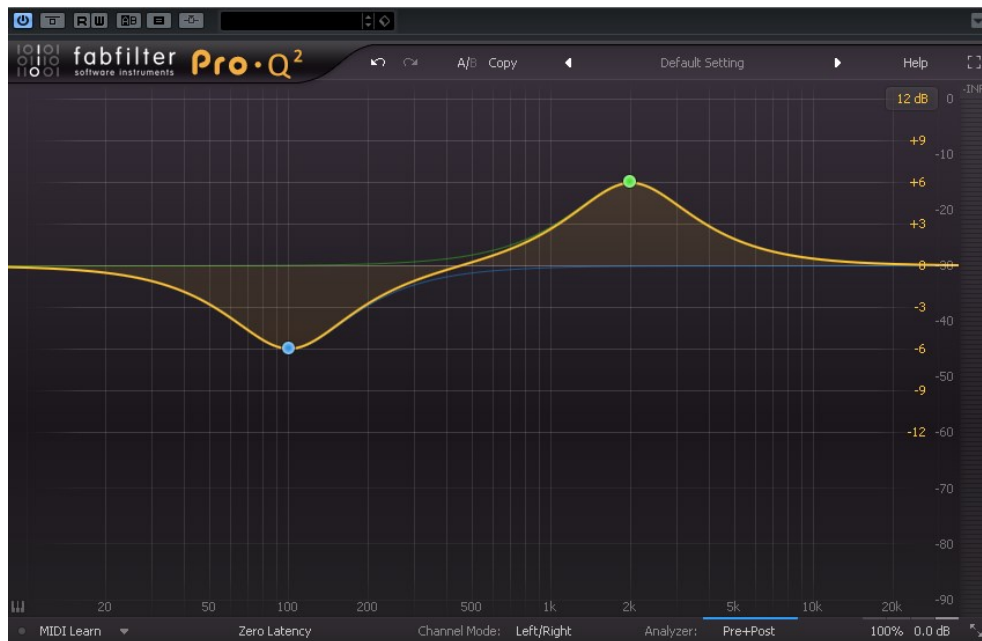
Figure 6: two Full Parametric Peak EQs set at 100 Hz (-6 dB cut) and 2 kHz (+6 dB boost), both with Q set to “1” – FabFilter ProQ2
