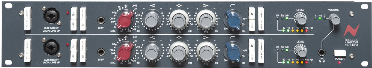
Figure 11: NEVE 1073 DPX Equalizer (analog hardware)
