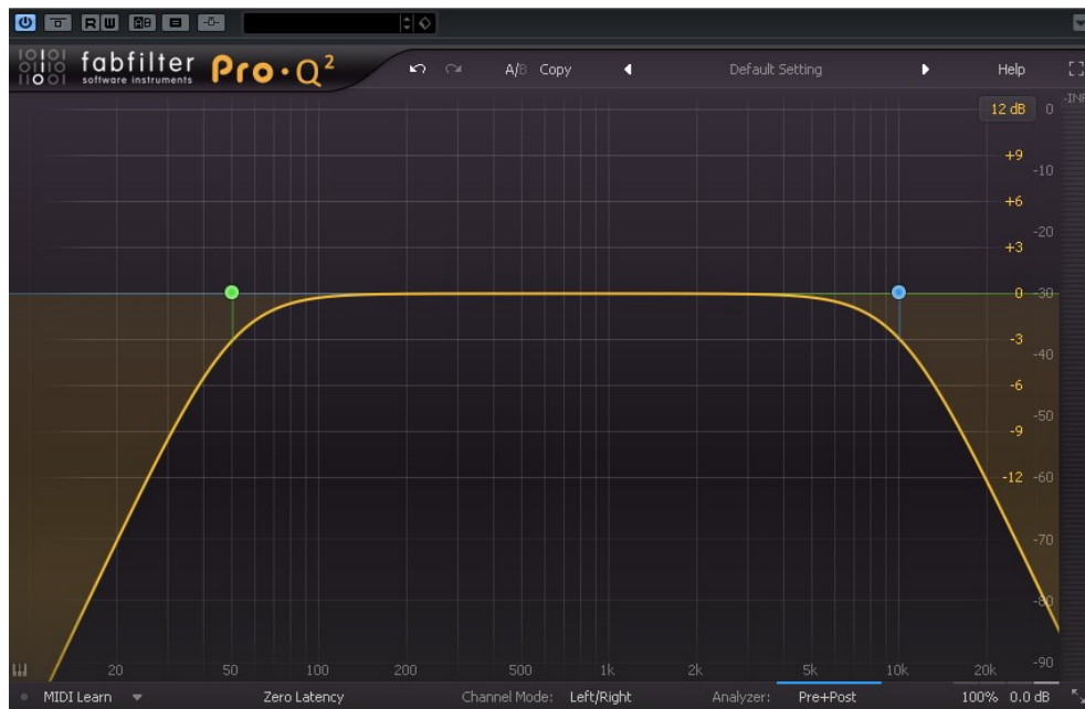
Figure 7: Low Cut filter set at 50 Hz and High Cut filter set at 10 kHz – FabFilter ProQ2
