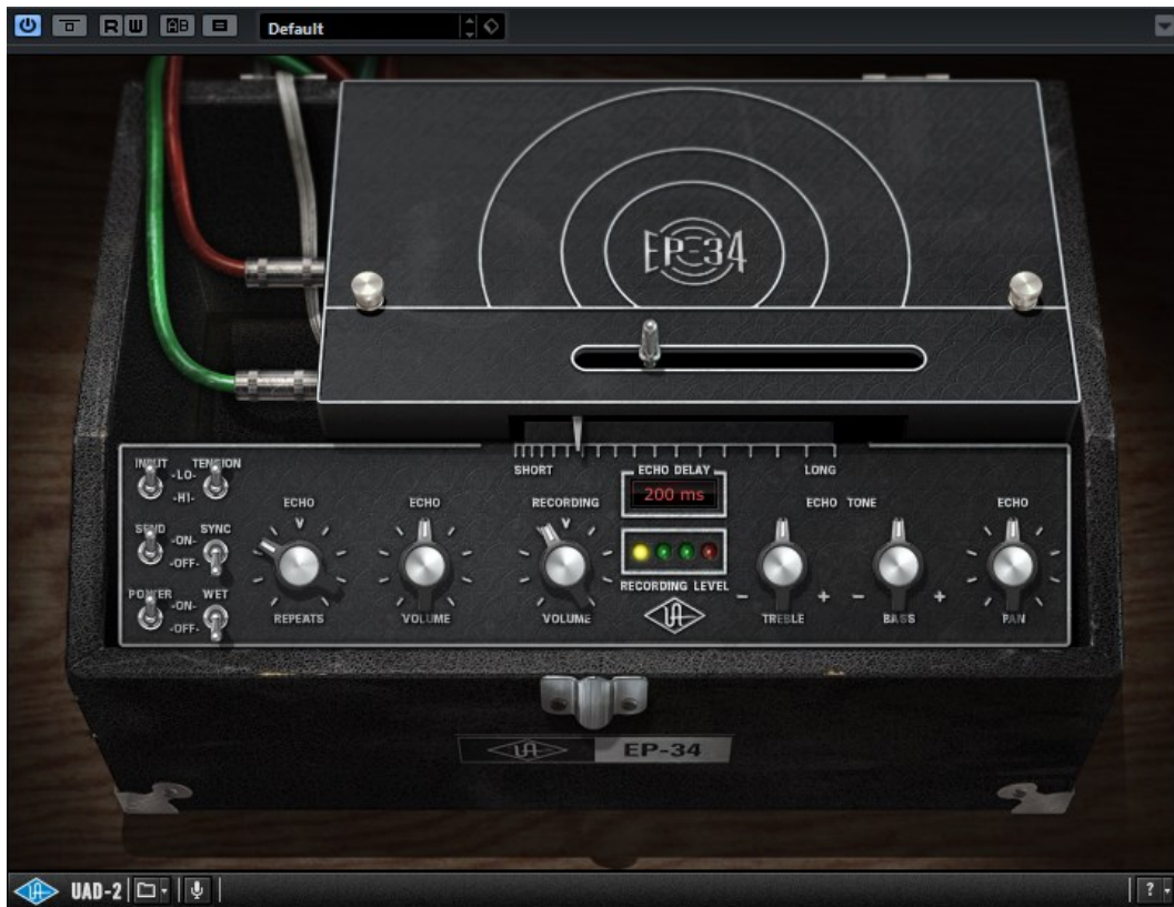
Figure 51: UAD EP-34 Classic Tape Echo (plugin, emulating the original Echoplex EP-3 and EP-4 hardware units)
