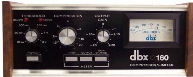
Figure 19: DBX 160 VCA-Compressor (analog hardware)
