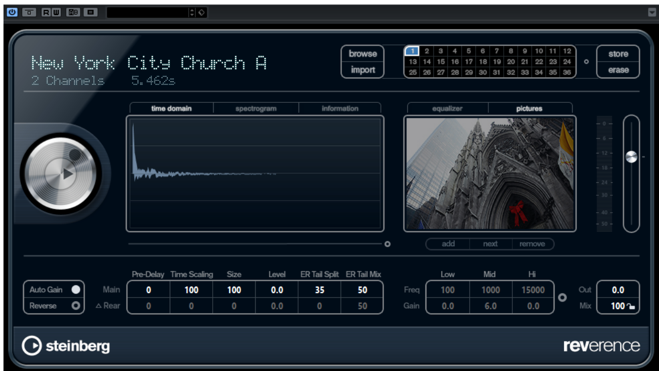
Figure 44: Steinberg REVerence Impulse Response Reverb (plugin, based on impulse responses recorded in real acoustic spaces)
