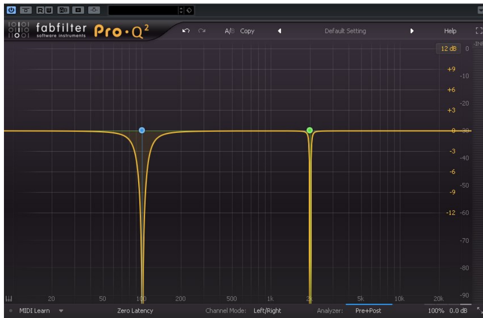
Figure 8: a Notch EQ set at 100 Hz (with Q set to a moderate 5) and another Notch EQ set at 2 kHz (with a much narrower Q of 40) – FabFilter ProQ2
