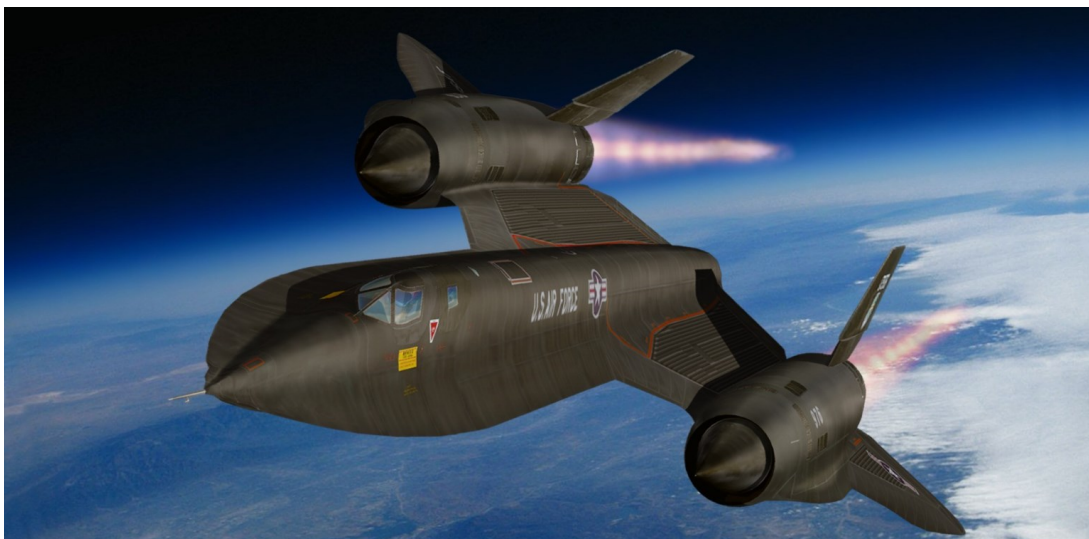
Figure 12: The Lockheed SR-71 Blackbird, the fastest jet aircraft ever built (in service between 1966 and 1999), that could travel up to Mach 3,3 (= 3,3 times the speed of sound, about 3.600 km/h)
