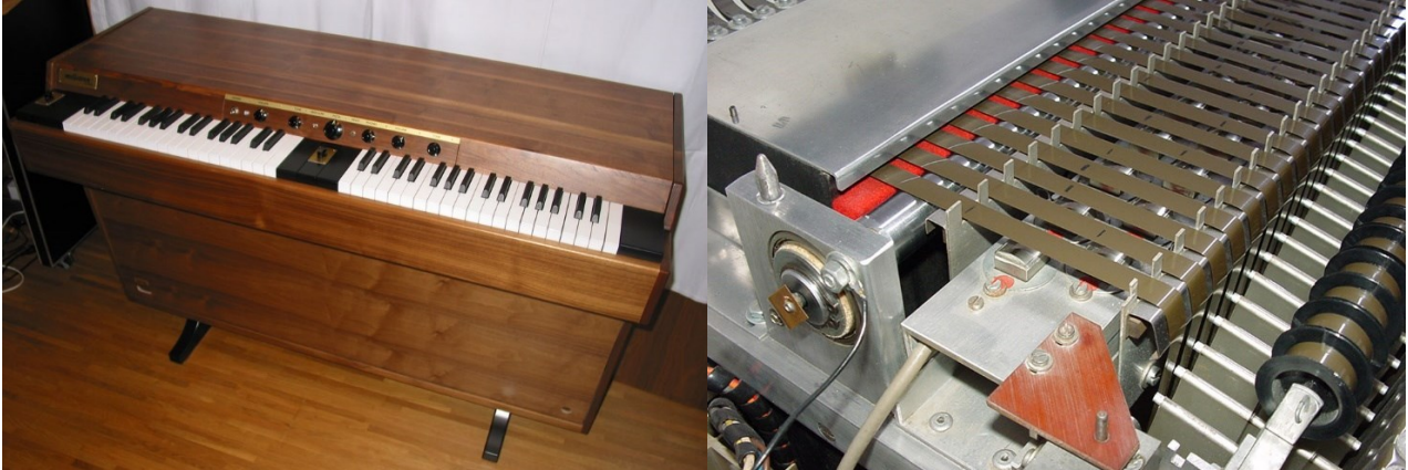
Figure 3: Mellotron Mk VII and internal tape-based playback system
